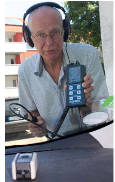
Ultrasonic leak detector USM 20128, with modulating transmitter (front) in the car interior.
