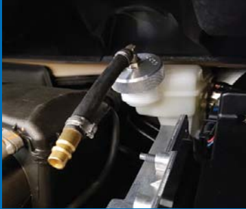
New cars: It's hard to reach the expansion tank. New angle adapters are essential.
