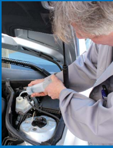
The expansion tank is emptied in no time at all.
