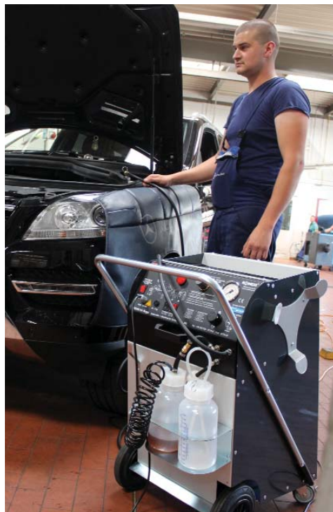
One unit of the RoTWIN generation for shop use: It meets the highest requirements, as it can also completely vent and bleed modern brake systems.
