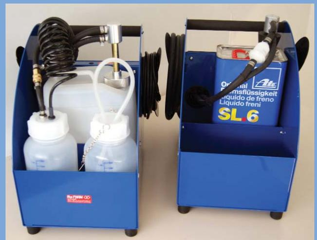
This is practical: the BW 1408 RoTWIN delivers the brake fluid from a commercially available five-liter container (right) as well as a transparent tank, which can be used for smaller brake fluid containers.
