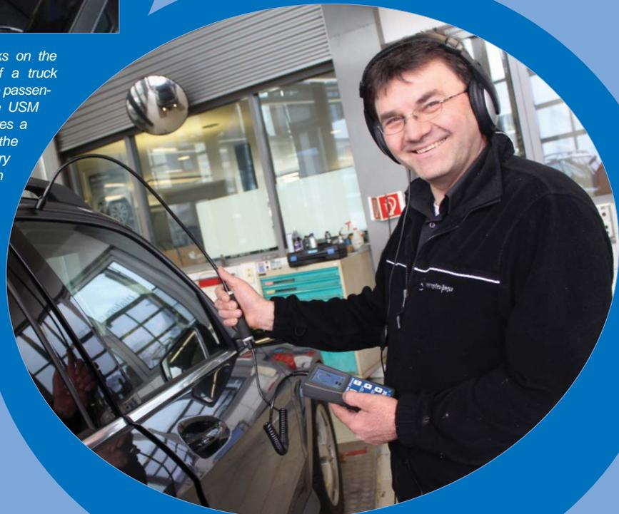
Leakage test of the passenger cabin with additional mod. transmitter (order no. 20128-S)
