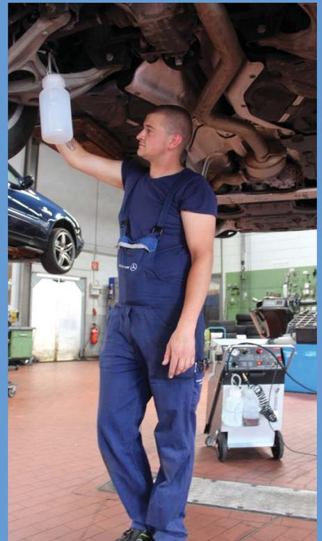
Different conditions apply today when changing brake fluid. The service unit must overcome higher resistances in the hydraulic treatment of modern brake systems.
