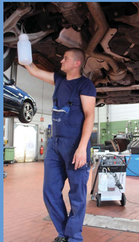
Different conditions apply today when changing brake fluid. The service unit must overcome higher resistances in the hydraulic treatment of modern brake systems.
