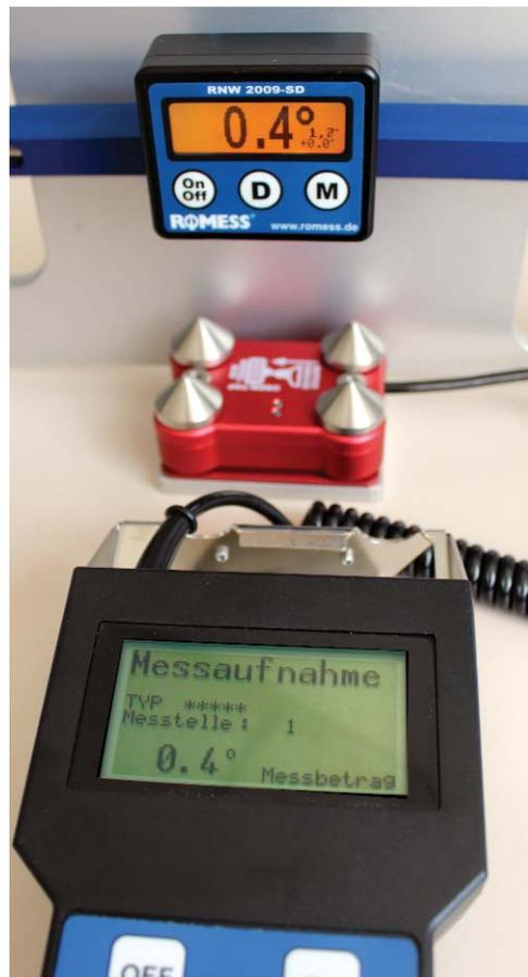
The test with the inclinometer in the aluminum base plate shows: The RNW 2009 balances the horizon automatically. Here and there the identical value is measured and off-set during a measuring procedure.
