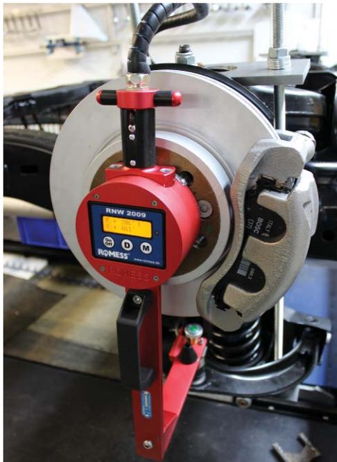
*The ROMESS measuring device 09860 accelerates the band production extremely fast and accurately.*
