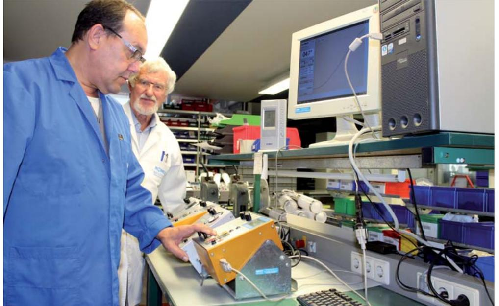
To ensure that they operate reliably and with high precision, the AQUA Series brake fluid testers are carefully adjusted during production.
