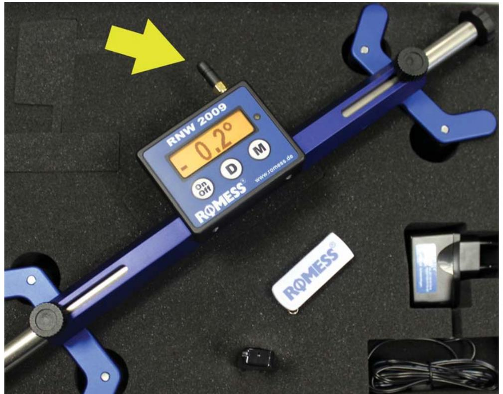
The steering wheel balance RNW 2009 Wireless (recognized by the antenna; see yellow arrow): The measurement data transmits with highest reliability from the vehicle to the measuring computer.
