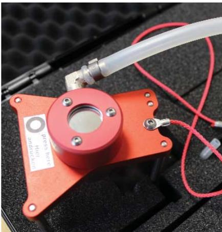
The DISTRONIC adjustment device of the latest generation is also available with reflector.
