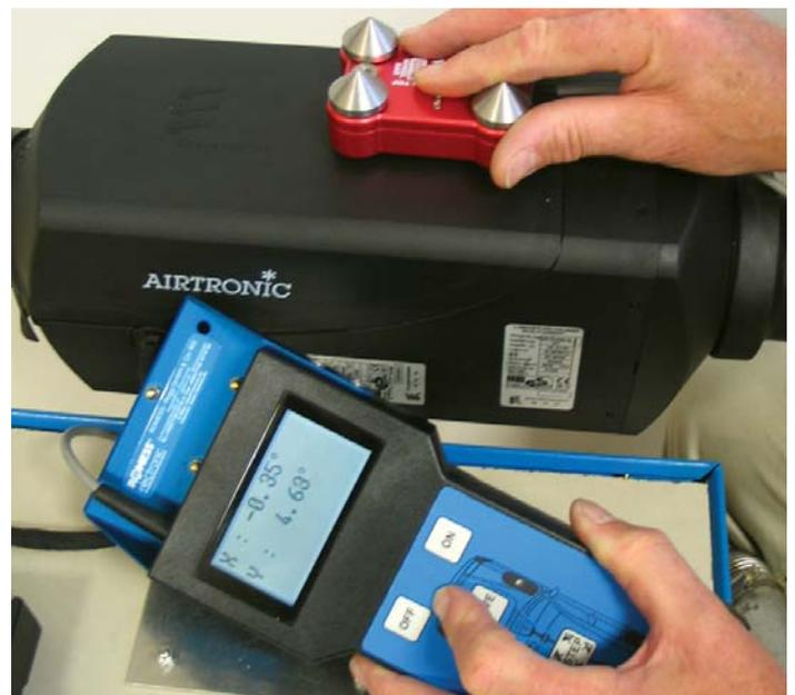
*The new biaxial angular measuring device 09709-10 is the ideal solution to guarantee the correct installation of vehicle heating systems.*
