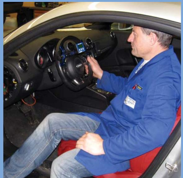
At the Robert Bosch school prospective master mechanics and technicians are shown by means of ROMESS devices how the professionals adjust the steering wheel during the wheel-alignment process.
