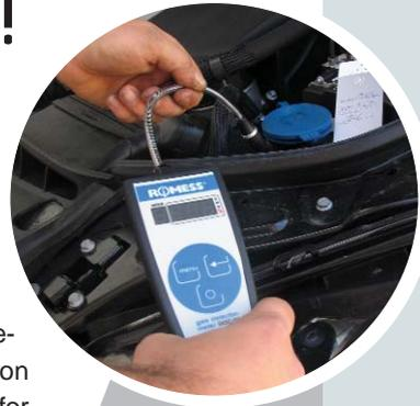
Application of the gas-concentration detecting device SKSC-01 (round picture). The handy test unit detects gases for example LPG (liquefied petroleum gas) or ethyl alcohol. The USM 2015 (right) is a technically well-proven ultrasonic leak-detecting device which locates any leakage at pneumatic braking systems of commercial vehicles as well as air conditioning in a fast and easy way.
