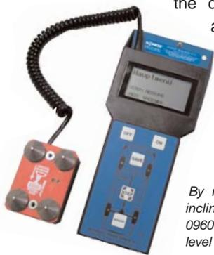
By means of the inclinometer CM-09606 the vehicle level is determined.
