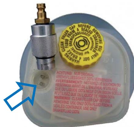
Perfect: Often a bayonet closure (arrow) is fixed on the reservoir of the VW and Audi models. This bayonet closure is usually covered by a small yellow cap. The ROMESS adapter 50201 has to be connected here.
