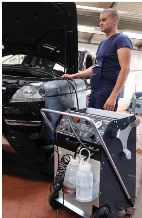
*One unit of the RoTWIN generation for shop use: It meets the highest requirements, as it can also completely vent and bleed modern brake systems.*
