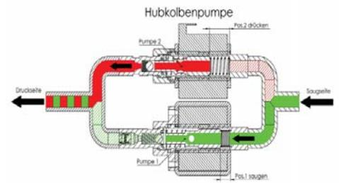
are alternately controlled (top). While one pump sucks, the other pumps the liquid further. This is the basis for the superiority of this worldwide patented system. Thanks to this innovative pump hydraulics, **modern brake systems can now be fully vented, which is no longer possible with conventional, simple service units.** This has been shown not only in shop use, but also tests carried out by, among others, demanding
