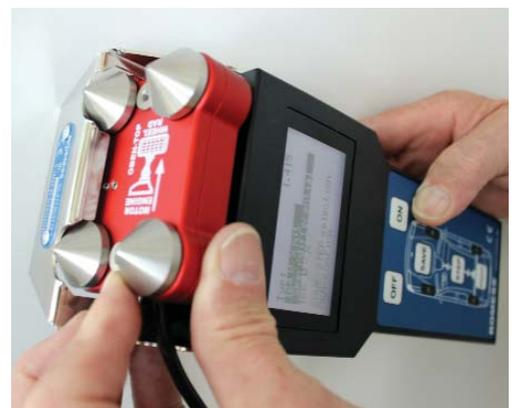
*Wheel alignment can be so simple: the CM 09606 inclination gauge is extremely practical.*
