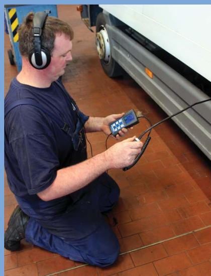
Air, steam and gas leaks with fissures of just below to 0.1 millimeters can be localized accurately.
