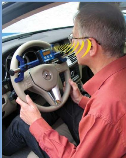
The device helps the automotive specialist even if the customer complains about uneven tire wear, although the suspension has been adjusted. The precise measurement results also allow a clean basic default setting of the chassis. The device has self-diagnostic capability and thus meets QM conditions.
