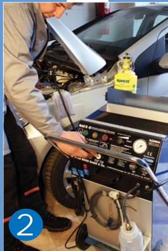
**3** The collection bottle with hose is attached to the ventilation nipple, and opened.
