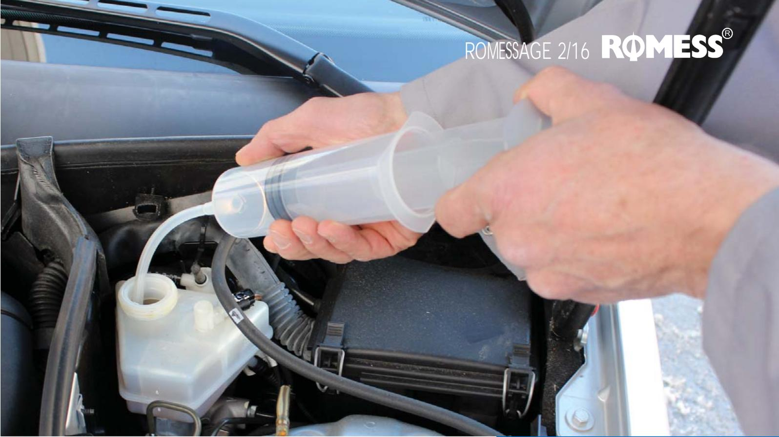
The ideal accompaniment for ROMESS devices without pre-drainage, with extremely high suction: our withdrawal syringe.
