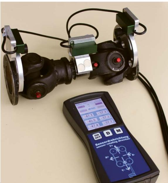
Experimental design, with the SL 2016 and a modified propeller shaft drive, as it is installed in heavy vehicles.
