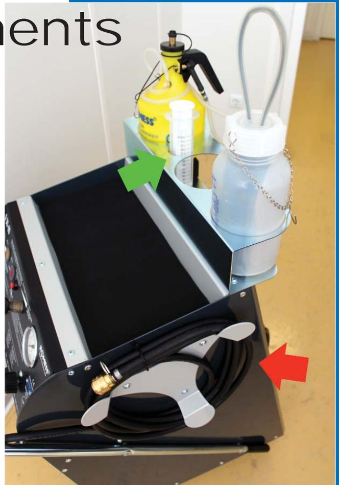
The ROMESS devices which do not accommodate a pre-drainage system will not have a fitting for the withdrawal syringe (green arrow). The S 30-60 (picture) has also a new elegant hose holder
